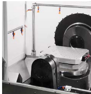
Wash down system
